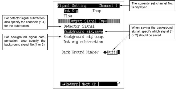
Fig. 16.6.7 Detector signal setup screen
