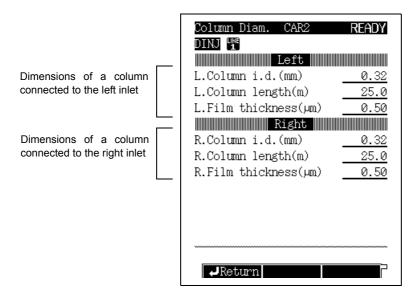
Fig. 12.1.4 Column parameters entering screen
