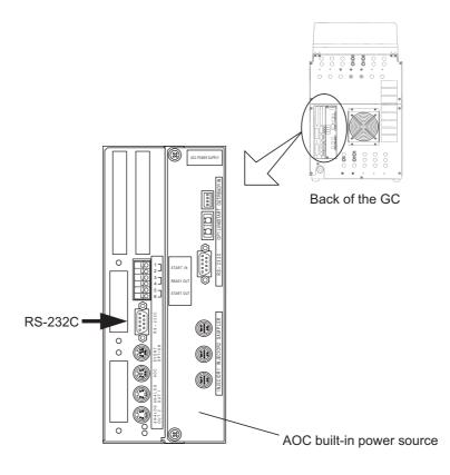
Fig. 2.3.1 Connection of RS-232C cable
