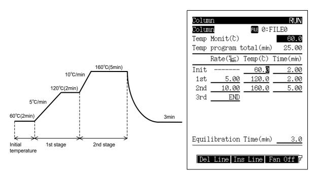
Fig. 11.2.2 Temperature program (Example 2)
