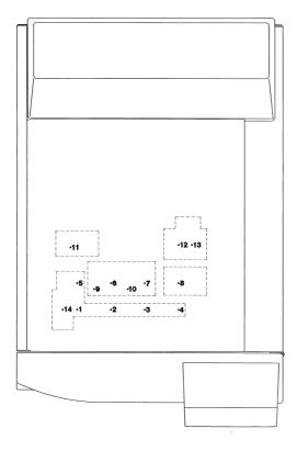
Fig. 4.1.1 Installation location for injection ports/detectors for capillary columns (layout viewed from the top of the unit)
