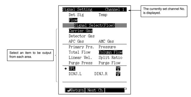
Fig. 16.6.9 Carrier gas signal setup screen
