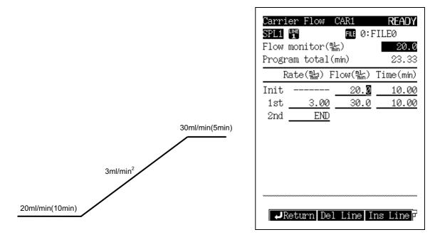
Fig. 12.2.11 Flow rate program example
