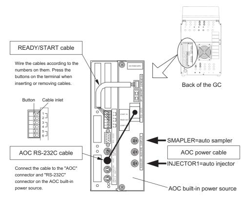
Fig. 2.5.1 Connection of the AOC-20 series
