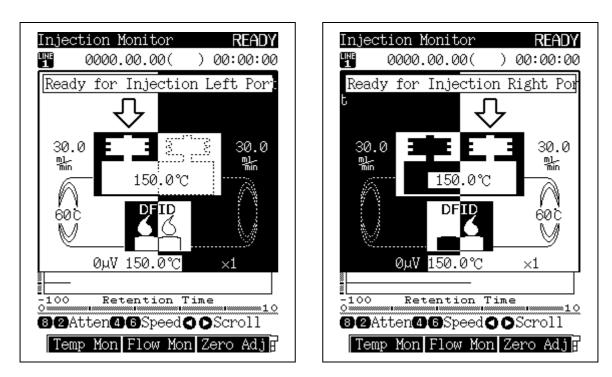
Fig. 10.1.1 Monitor injection screen
