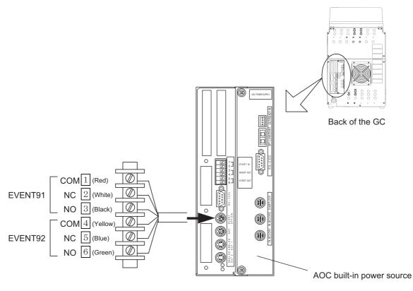
Fig. 2.6.1 Connecting a relay cable
