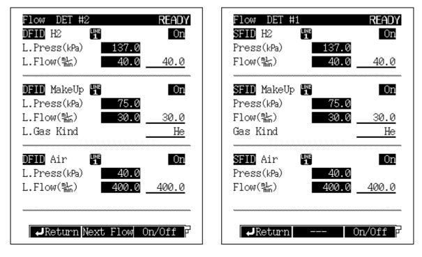
Fig. 13.1.5 Setting the detector gas flows
