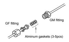
Fig. 1.3.2 Joining Type G fittings
