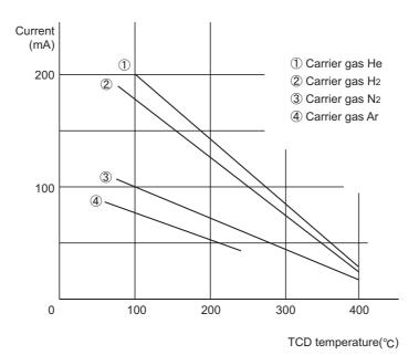
Fig. 13.2.3 Maximum operating current
