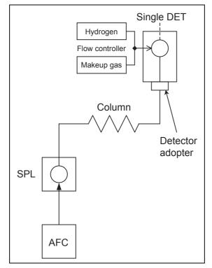
Fig. 4.5.1 Single DET (In case of FID)
