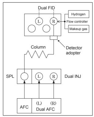
Fig. 4.3.1 Dual FID (flow controller)
