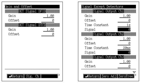
Fig. 16.6.13 Detector signal gain and offset screen
