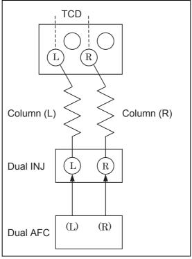
Fig. 3.4.1 Dual-column configuration (TCD)
