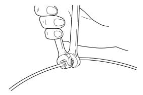
Fig. 1.3.3 Tightening the joints
