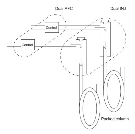
Fig. 12.1.1 Dual-column packed analysis
