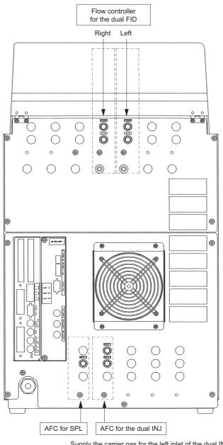
Supply the carrier gas for the left inlet of the dual INJ to CARRIER L and the carrier gas for the right inlet of the dual INJ to CARRIER R.
