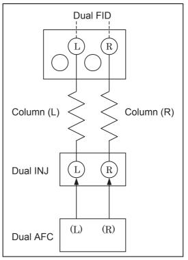
Fig. 3.2.1 Dual-column configuration
