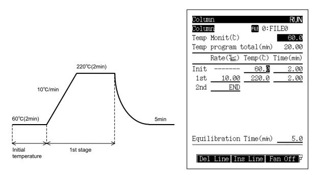
Fig. 11.2.1 Temperature program (Example 1)
