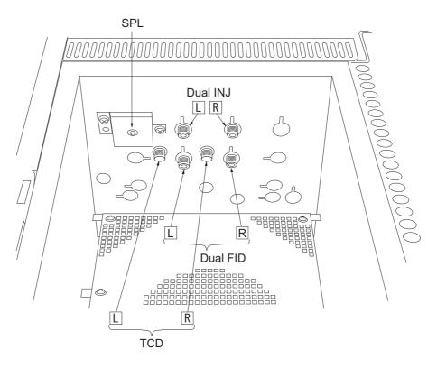
Fig. 3.1.2 Column connecting joints (GC-2014ATF+SPL model)
