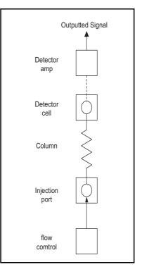
Fig. 2.1.1 Concept of analytical flow lines
