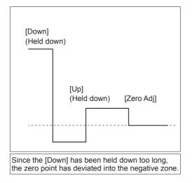
Fig. 9.4.1 Zero point adjustment
