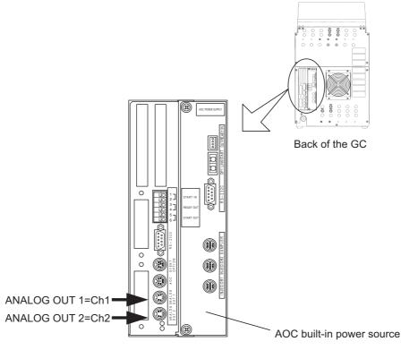
Fig. 2.2.1 Connecting the Chromatopac signal cable
