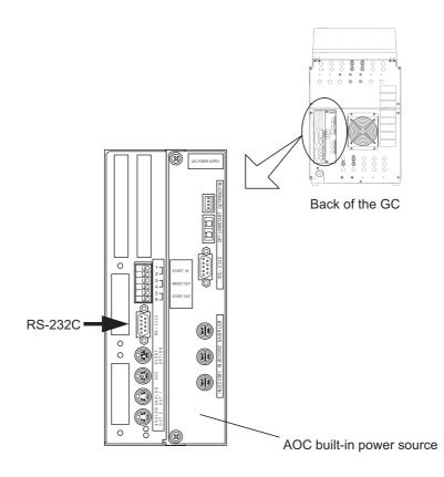
Fig. 2.4.1 Connection of RS-232C cable
