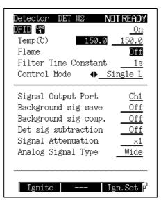
Set to "Single L" when the column is connected to the left (L) side of the dual FID and "Single R" when it is connected to the right (R) side.
