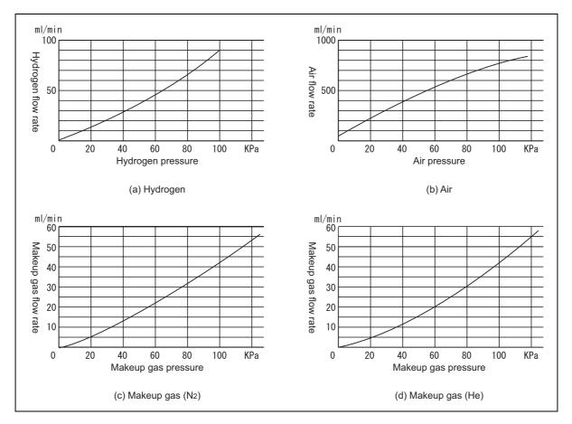
Fig. 13.1.4 Pressure-flow rate calibration curves (examples)
