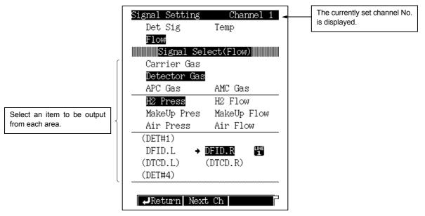
Fig. 16.6.10 Detector gas signal setup screen
