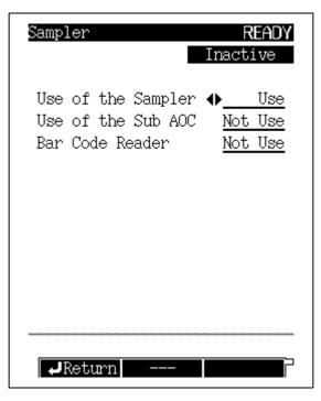
Fig. 15.1.4 Sampler carousel and other options setup
