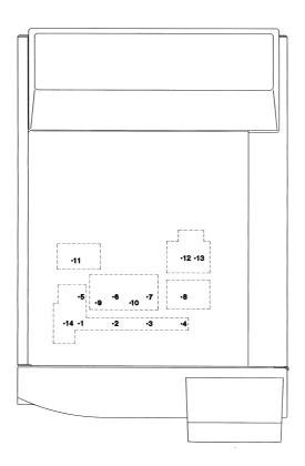
Fig. 3.1.1 Fig. 3.1.1 Installation location for injection ports/detectors for packed columns (layout viewed from the top of the unit)
