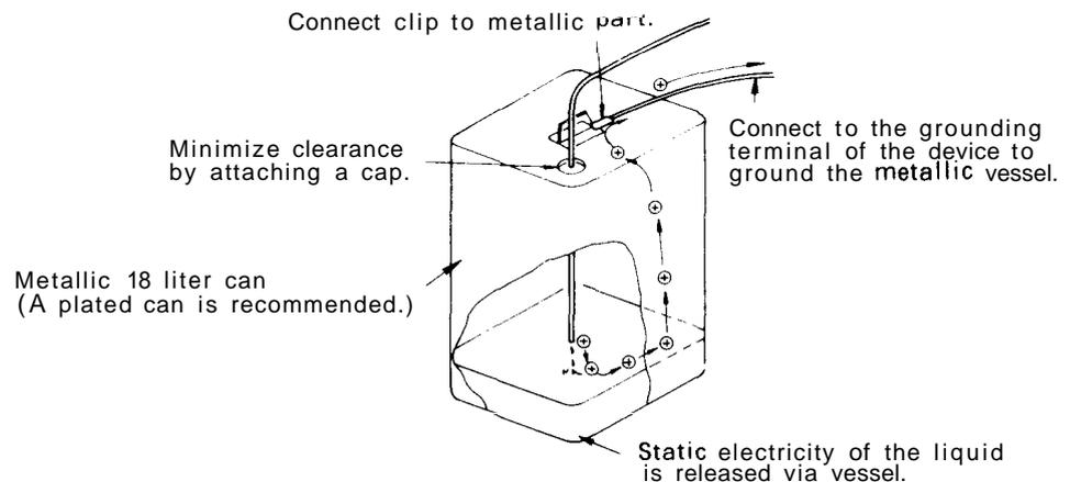
**Fig. 12.3 Anti-Static Electricity Measures for Vessel**
