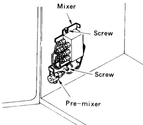
(B) Mounting on the inside right wall (In contrast with mounting it on the left side, the mixer is mounted upside down.)
