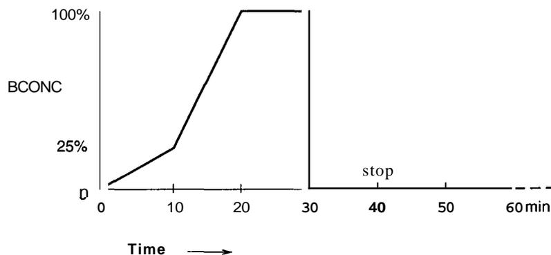
Note that the concentration delivered at any given time is based on a linear interpretation of proportionality between each defined point. (Nonlinear curves are available by control with the SCL-10A.)
