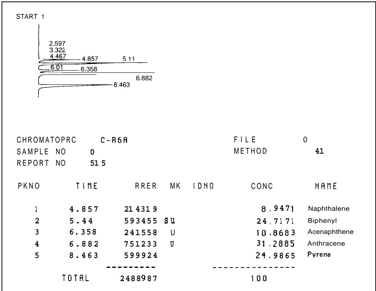
The concentration of each solvent in high pressure gradient elution can be tested without a column or sample in the following method.
