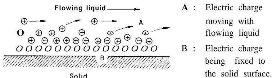
A : Electric charge moving with flowing liquid
